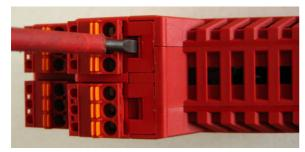
2. Using the screwdriver, push the splint down from the locked closure tab
