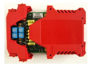
4. You can now open the LVCpro and the code-switches for the adjustment and/or calibration of the press force are accessible.
