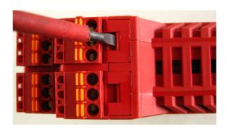
1. Use a screwdriver to push the splint in the opening tab down, located underneath the connector plugs of Power, PiezzoSensor2 and underneath PeakOut2 and AnalogOut2.
