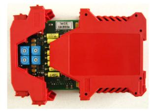
4. You can now open the LVCpro and the code-switches for the adjustment and/or calibration of the press force are accessible.
